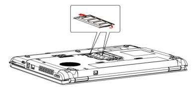
Figure 8-8 Removing the memory module
